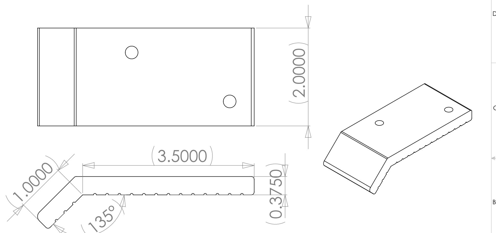
6061 T6 Aluminum. Debur. Type II Clear anodize or Hard Anodize.
